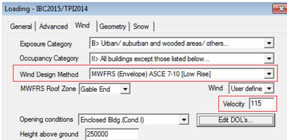
Since the 2012 IRC wind speed map is based on a “nominal” wind speed, but the wind speed entered into MiTek Engineering must be an “ultimate” wind speed as found in the references noted above, the program reports the ultimate design wind speed ( $V_{ult}$ ) along with the nominal design wind speed ( $V_{asd}$ ) when ASCE 7-10 is chosen.
